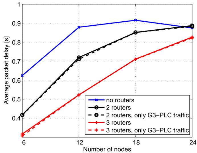
Figure 2.4: End-to-end delay for the energy management network.
